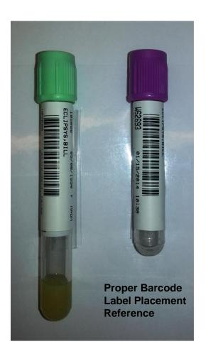
Proper barcode label placement has the following characteristics:Label and barcode placed as close to the colored stopper as possible
